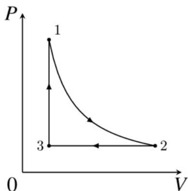
$$Q_{31} = vC_V(T_3 - T_1), \quad Q_{23} = vC_p(T_2 - T_3) = -vC_p(T_3 - T_1). \quad \frac{T_1}{T_3} = \frac{T_2}{T_3} = 3.$$
